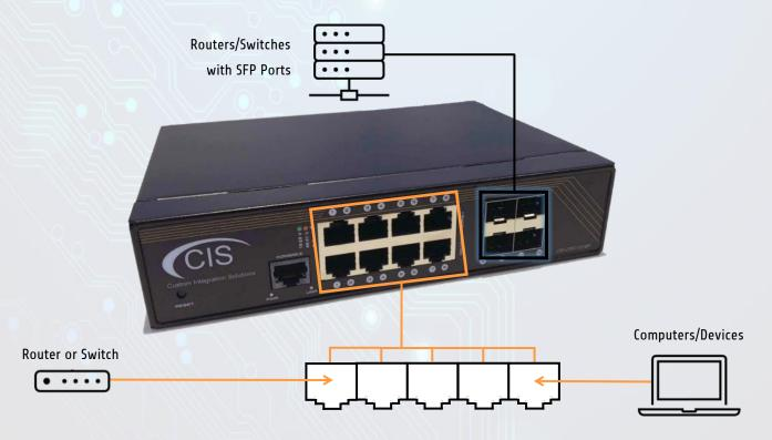
Connect your router or upstream switch to any of the Ethernet ports, or use an SFP connection if your device supports it. Connect your devices to the remaining ports
