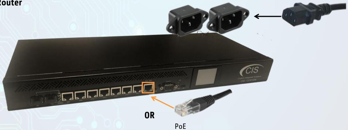
Connect a power cable to the rear of the device, or use PoE in on ETH7 labelled “PoE/Boot.”
