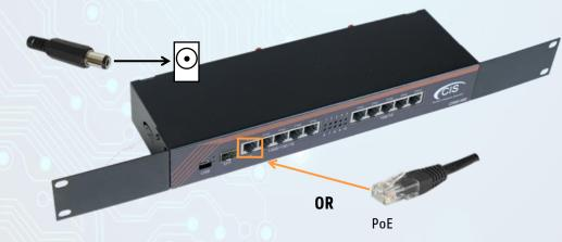
Connect the included power supply to the DC jack on the rear of the device, or power via PoE on ETH1
