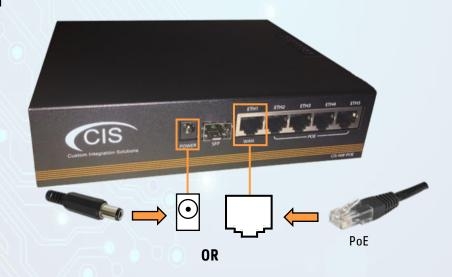
Connect the included power supply to the DC jack on the front, or power via passive PoE on ETH1
