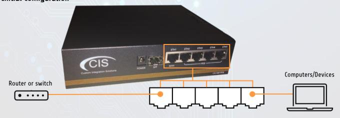
Connect your router or upstream switch to any of the Ethernet ports. We recommend you use the first or last port, and stay consistent in your installations to make troubleshooting easier. You must use the first port if you wish to power the switch via PoE. Connect the remaining ports to your devices.
