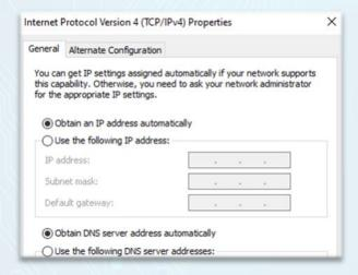
2. Obtain the IP Address of the **Default Gateway**. CIS Routers use **10.100.1.1** as the default. You can open a **command prompt** on a Windows machine and enter **ipconfig** to get the default gateway.
