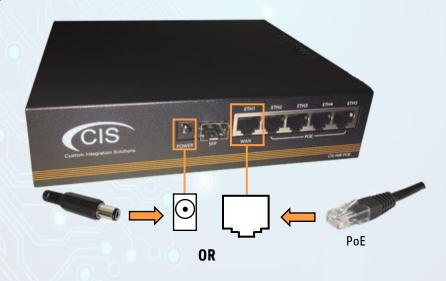
Connect the included power supply to the DC jack on the front, or power via passive PoE on ETH1
